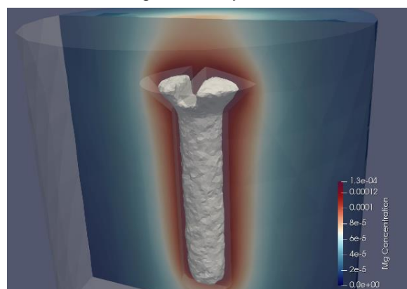
Fig 1. Simulation result of Mg 2+ ions release (ion concentration in g/mm 3 ) and biodegradation of a simple screw
